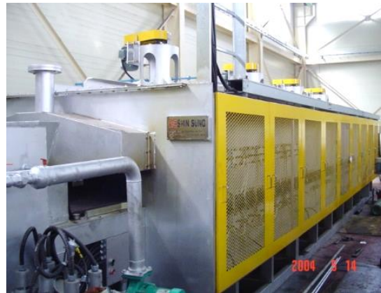
5. HEAT TREATMENT FURNACE OUT SOURCING
